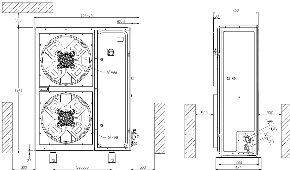
Figure 16: Dimensions of ZXDI condensing units (all models)
