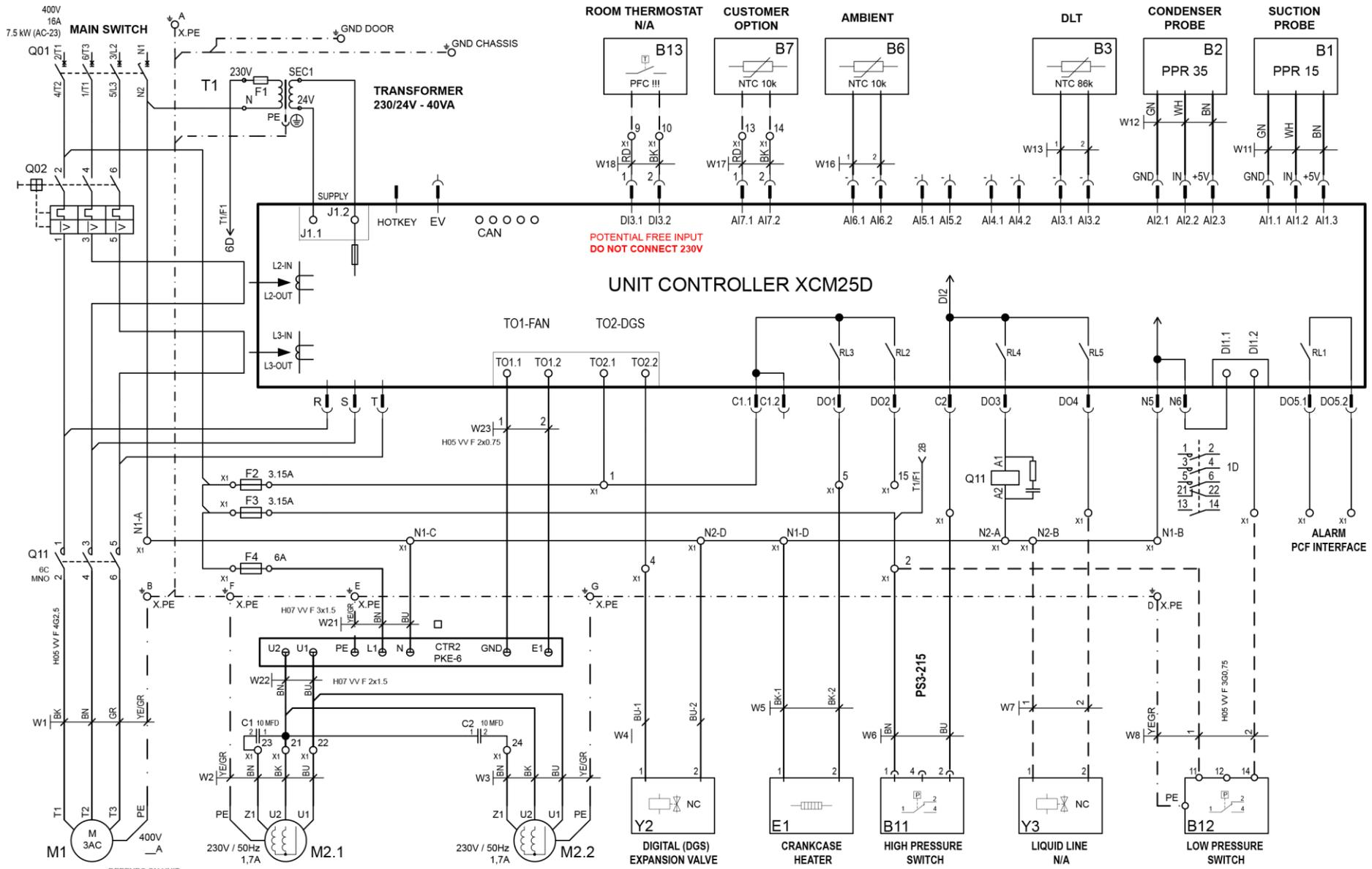
**Figure 24: Wiring diagram – 3-Phase motor**
