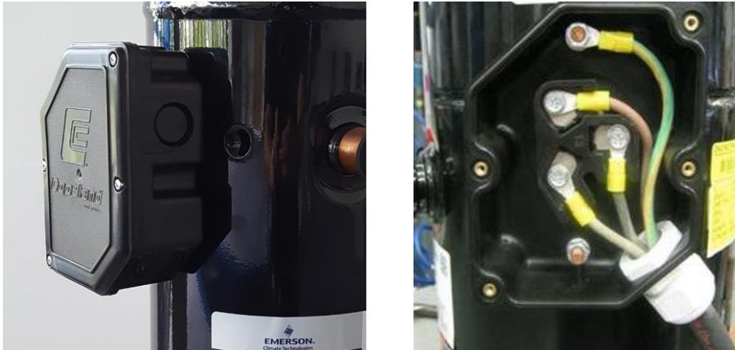
Figure 26: IP54 T-Box and correct electrical installation with cable gland
