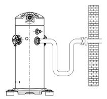
Under some conditions, the Copeland scroll has a normal starting rotational motion that can transmit a transient noise along the lines. This may be particularly pronounced in compressors using a three-phase motor due to their inherently higher starting torque. This phenomenon, like the one described previously, can easily be avoided by using standard line isolation techniques.
