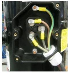
Figure 16: IP54 T-Box and correct electrical installation with cable gland
