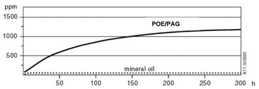
Figure 22: Absorption of moisture in POE/PAG oil in comparison to mineral oil in ppm by weight at 25  $^{\circ}$ C and 50  $^{\circ}$ C relative humidity (h= hours)
