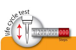
As envisaged by the CAREL product development procedure, E<sup>3</sup>V-C has also been lifetime tested, confirming reliable operation even after 1.2 billion steps performed in limit operating conditions.
