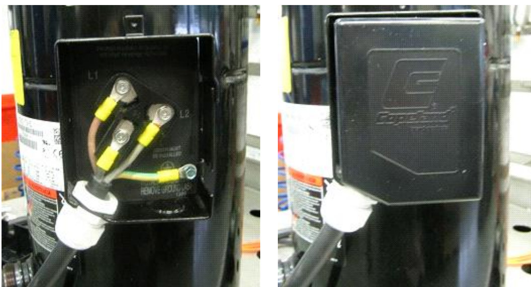
Figure 29: Correct electrical installation with cable glands for IP21 T-box
