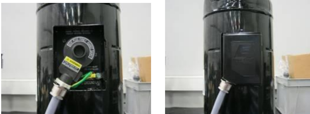
Figure 21: Terminal box IP66 and correct electrical installation with cable glands
