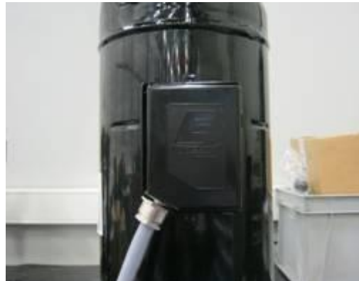
Figure 21: Terminal box IP66 and correct electrical installation with cable glands
