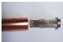
The filter screen should be placed into the small tube running at 90° to the solenoid valve stem. A narrow washer fixed on the filter screen will sit on the end of the tube preventing it from falling inside (see photos). The tube running from the top centre of the compressor down to the previous tube needs to be swaged at the solenoid valve end so that it covers the filter screen/tube and is then brazed into position.
