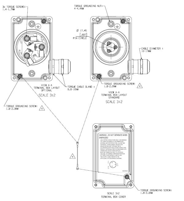
Figure 10: Cable gland torque and diameter and electrical connections torque
