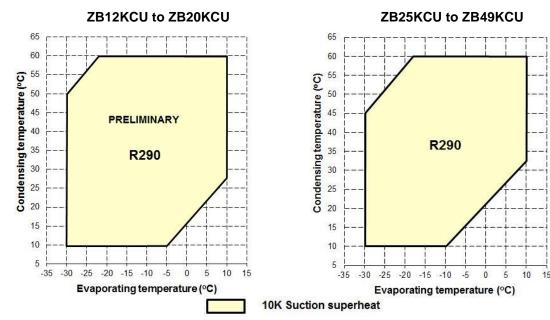
Figure 1: Application envelopes for compressors ZB12KCU to ZB49KCU with R290 C6.2.28/0915/E
