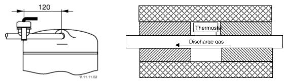
Figure 12: Example of installation of an external discharge gas temperature protection
