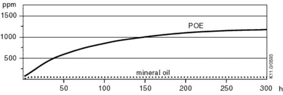
Figure 15: Absorption of moisture in ester oil in comparison to mineral oil in ppm by weight at 25° C and 50% relative humidity (h=hours)
