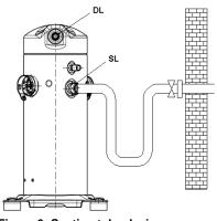
Figure 6: Suction tube design
