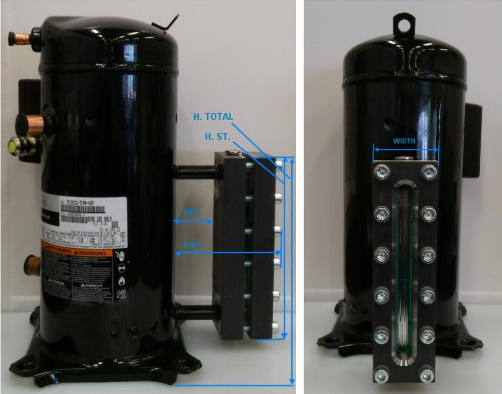
Figure 13: Sample compressor equipped with a level glass
